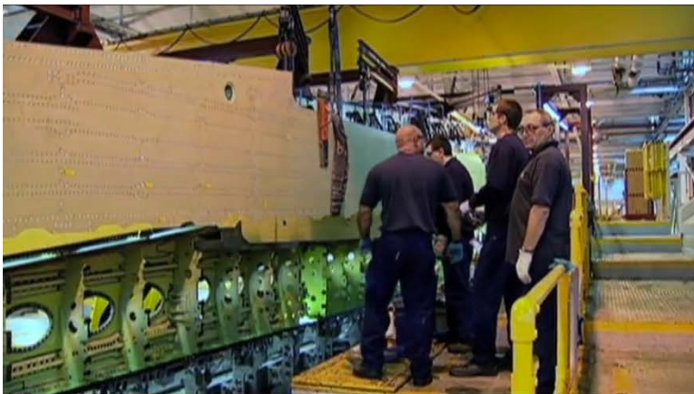
Workers align aluminum skin with wing assembly
